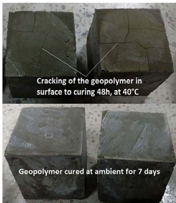
Fig. 4. Synthesized geopolymers ( 5 \times 5 \times 5 \text{ cm}^3 cubes).
